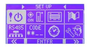
To prevent the set function from being modified, a password can be entered that must be input every time the digital programmer is used.
