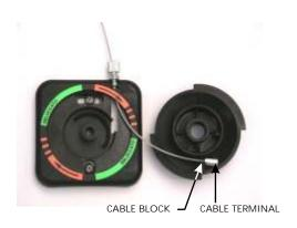
Pass the release cable in the slit in the base and then inside the adjustment register as shown in the figure. Then position the cable terminal on the release knob cable block (see figure).
