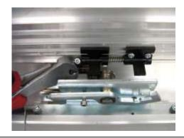
Turn the release knob to check system operation; turning the knob clockwise to a released position, the electric lock must free the leaves and when returning the knob to the blocked position, the electric lock must block the leaves again.
