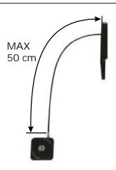
Identify the fastening point on the wall, considering that the standard cable sheath is 50 cm long.
