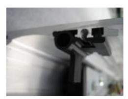
At this point, insert the plastic release components inside the specific slot made in the upper part of the crosspiece and check that they can slide freely in their housing without going out.
