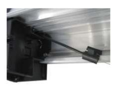
Insert the plastic release components as shown in the figure, considering that 4 plastic components are necessary to install the manual release on the left side.
