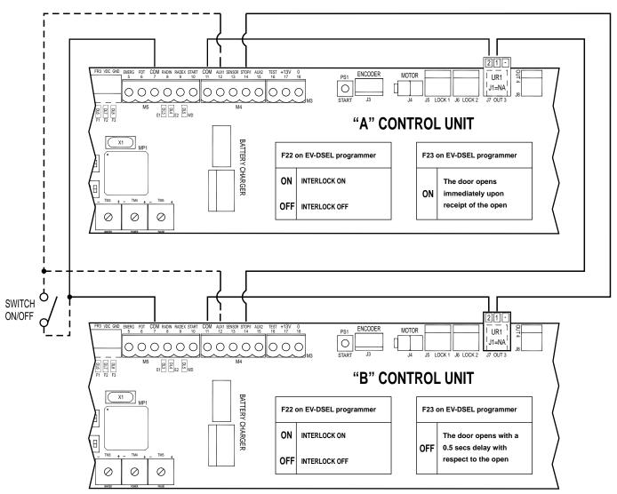
The dotted line of the ON/OFF switch connected to the AUX/1 input is used to disable the interlock operation (connection not essential for the system operation).
