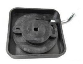
Insert the steel cable inside the bend pipe as shown in the figure.
