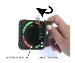
Now, insert the release knob on the base of the mechanism, being careful to keep the cable terminal in the seat of the cable block and the knob in the correct position. When inserting the knob, the cable terminal must be in the position just beyond the lower fastening screw, in a clockwise direction.
