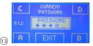
Press the button in correspondence of the letter "A" a fourth time, and an asterisk will appear on the display in the field for the fourth letter.
