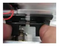
Position the second and third plastic release components as shown in the figure, making sure that the stroke of the third component is sufficient to activate the lever on the electric lock. Fasten the second component into position with self-threading screws.
