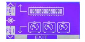
To set the functions relative to the dip switches, briefly press the F01 **F2** button (see paragraph 6a).
