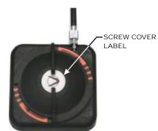
Apply the screw cover label on the fixing screw. By moving the release knob to the NOT RELEASED position, only the orange part of the label must be seen with the drawn black arrows.
