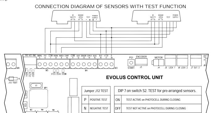
The diagram illustrates the connection on the operator of two sensors with twin outputs and monitoring test to detect movement (radar) and presence (safety photocell).
