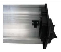
Fasten the first plastic release component near the right side panel with 2 of the self-threading screws in the kit, which will catch in the narrow slot on the crosspiece.
