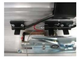
In order to keep the sheath in position, it is recommended to insert it in one of the automation's fairleads.
