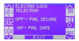
Press the station to go to the third setting required, "S03", relative to the automatism module: select OFF with the F1 button for an EVOLUS 90 model or ON with the F3 button for an VOLUS 150 model.
