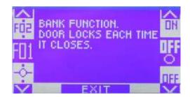
To change the status of a dip switch, press the ON  $\,$  **F3** button to set the dip switch to ON .
