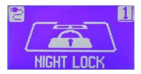
The door's automatic mode is deactivated and the leaves can be moved manually.
