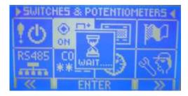
Press the **F1** button until the section that corresponds to the functions and settings is displayed and briefly press the ENTER (SET) button to access it.
