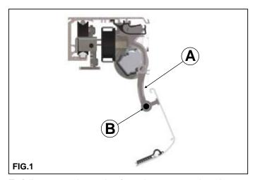
To fully remove the casing from the automated equipment press the end section of the pins (B) located on the support links and extract them by pulling them from the opposite end (Fig. 1)
