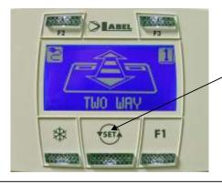
By pushing the central button select the automatic door work mode.
