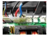
The electric lock kit includes a power supply cable. This cable has two wires on one end that are connected to the electric lock solenoid valve wires with the specific terminals. The other end of the cable has a connection that is inserted in the LOCK1 connector on the Evolus operator electronic control unit.
